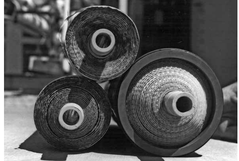
Reverse osmosis (RO) membranes
